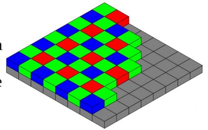
One of the main facilities of this sensor-type is the simultaneous observation of the star through four filters. It is especially interesting, that the two green layers gives two independent observations of the same star. The difference  $G2 - G1$  is a fine measure of how accurate the star is observed.
